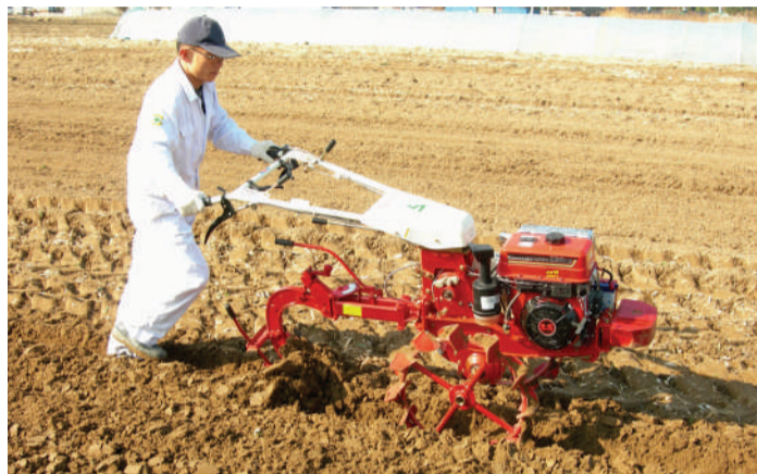
Plow (TP-25) - Moisture width: 26.5cm - Work volume: (0.66 or 1 Ha /day) 2000 pyeong/day
