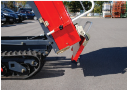
Automatic opening of rear door when dumping
