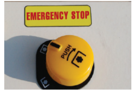
Emergency stop switch that can safely turn off the engine in emergency situations
