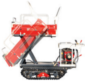
Dump and lift conversion with simple lever operation
